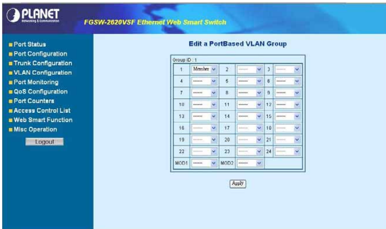
Figure 4-17 Edit Port-based VLAN Setting Web Page screen
